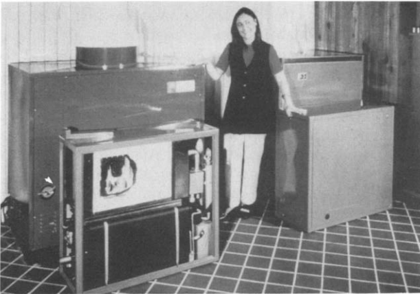
Fig. 4. 12.5 kW field test fuel cell by International Fuel Cells.
