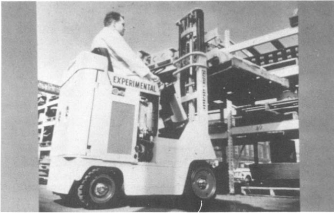
Fig. 1. Prototype fuel cell powered lift truck by Allis-Chalmers.
